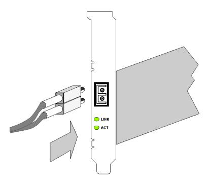
Figure 2. Connection of fiber-optics cables/plugs
